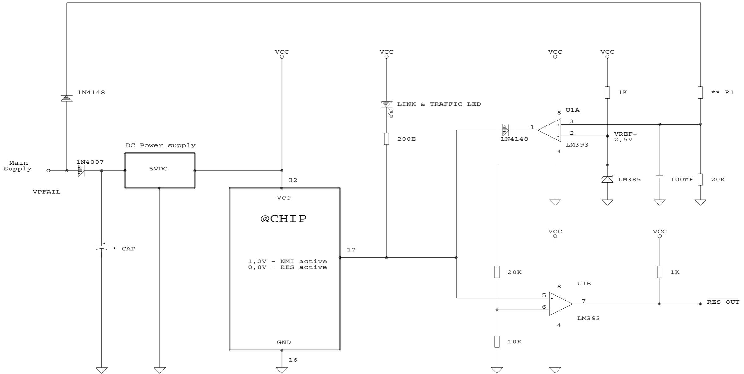
VPFAIL = Power Fail is used to monitor main supply voltage, not main Vcc+5VDC.
