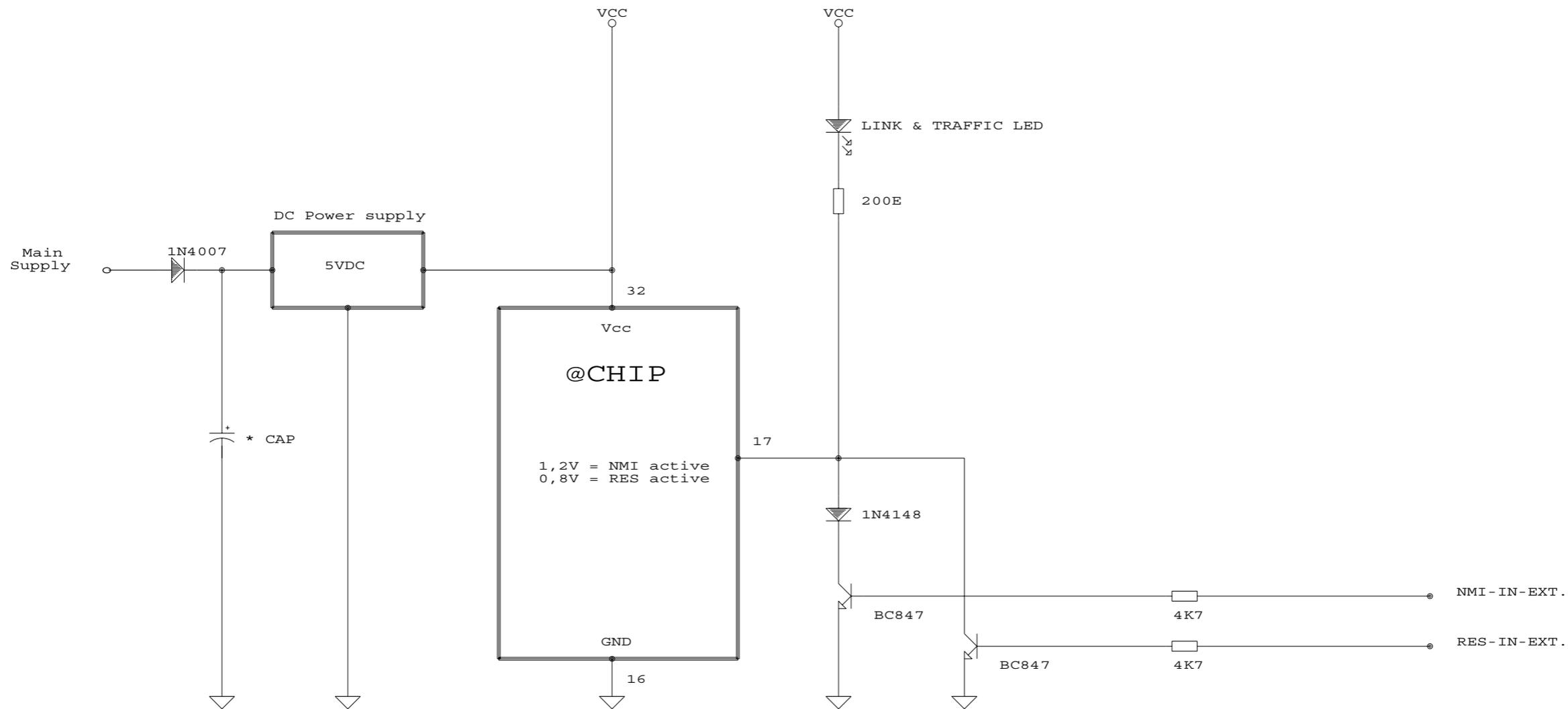
NMI-IN-EXT = High active digital NMI - Input from any external Logic.
